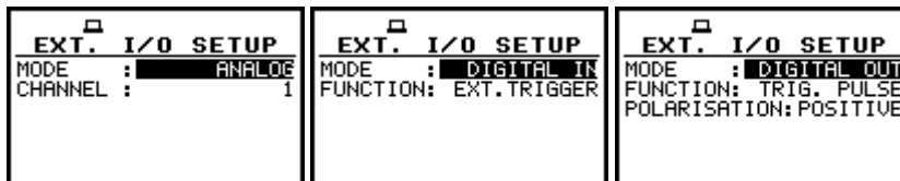
EXT. I/O SETUP windows with the different I/O devices selection
