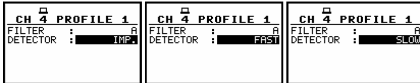
CHANNEL x PROFILE y windows (SM) with the selection of the RMS detector
