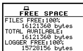
FREE SPACE window after the execution of the DELETE ALL operation
