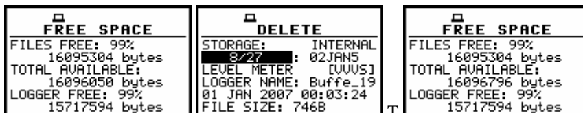
Execution of the 02JAN5 file deletion and the influence of this process on the memory space
