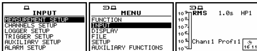
Displays after three consecutive pressing of the <ESC> push-button from MEASUREMENT SETUP window
