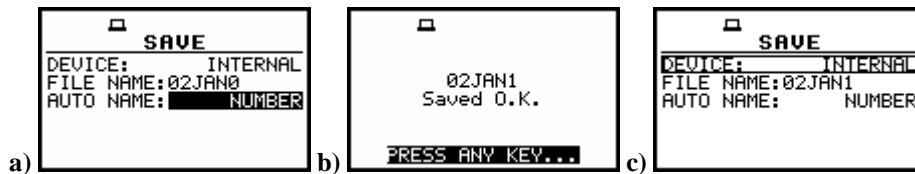
SAVE window AUTO NAME option selected (a), after saving the file with the increased name (b) and after repeated enter to SAVE window (c)
