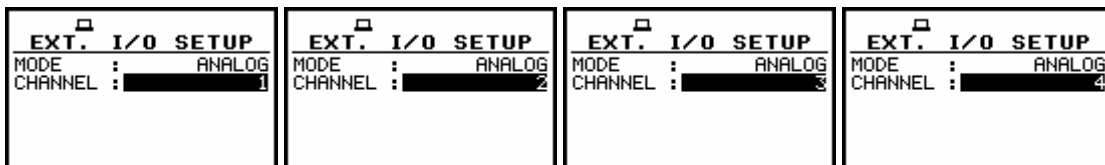
EXT. I/O SETUP windows with the channel selection for output signal
