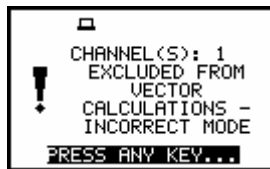
Display with the warning that CHANNEL x has been excluded from vector calculation
