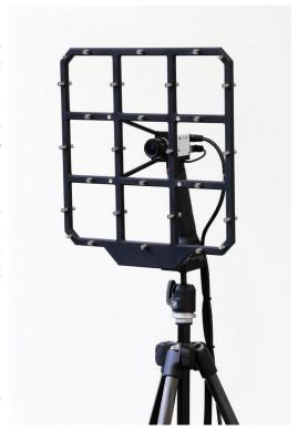
The design of the paddle allows for easy handling as it is lightweight and features cable bundling with one cable bundle holding 24 microphone channels.
