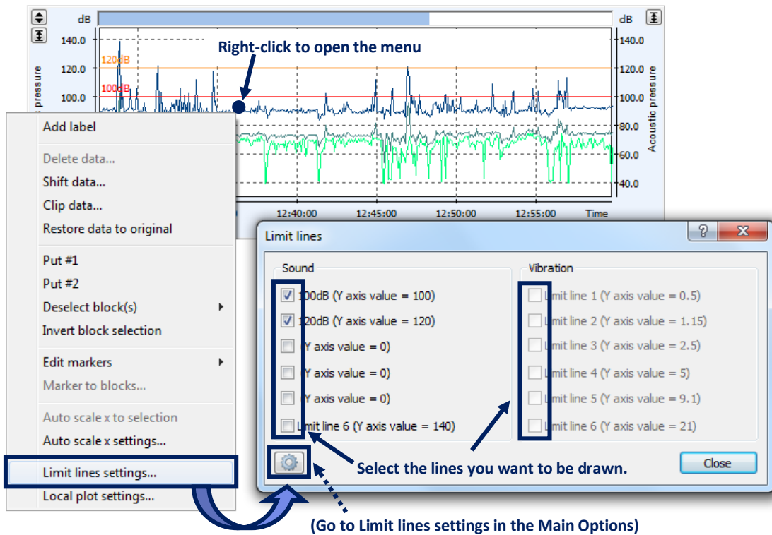
Fig. 4-51. Setting the visibility of limit lines on a plot
