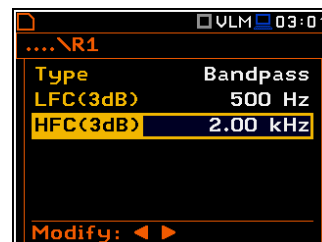
Selection of a wide and narrow Bandpass Real Time Filters
