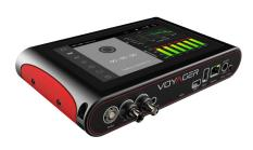
The success of the Scan & Listen device led to the development of Voyager that allows one to gain understanding about the sound field in addition to real-time visualization, listening and audio filtering. The embedded touch controlled software offers the ability to run targeted vibro-acoustic analysis intuitively on the spot. Monitor soundscapes and locate sound sources reliably over a broad frequency range with short, quick scans.
