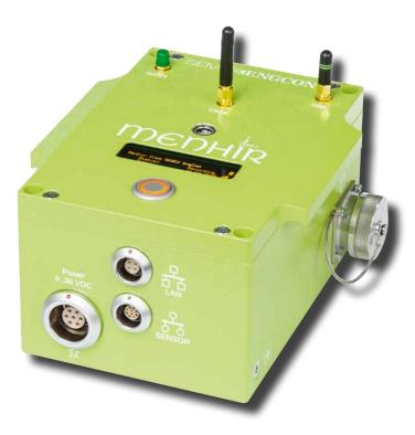
**MENHIR** is a robust and highly reliable seismic monitoring device that operates in network topologies to monitor seismic strong motion and quickly analyzes their impact on dam structures.
