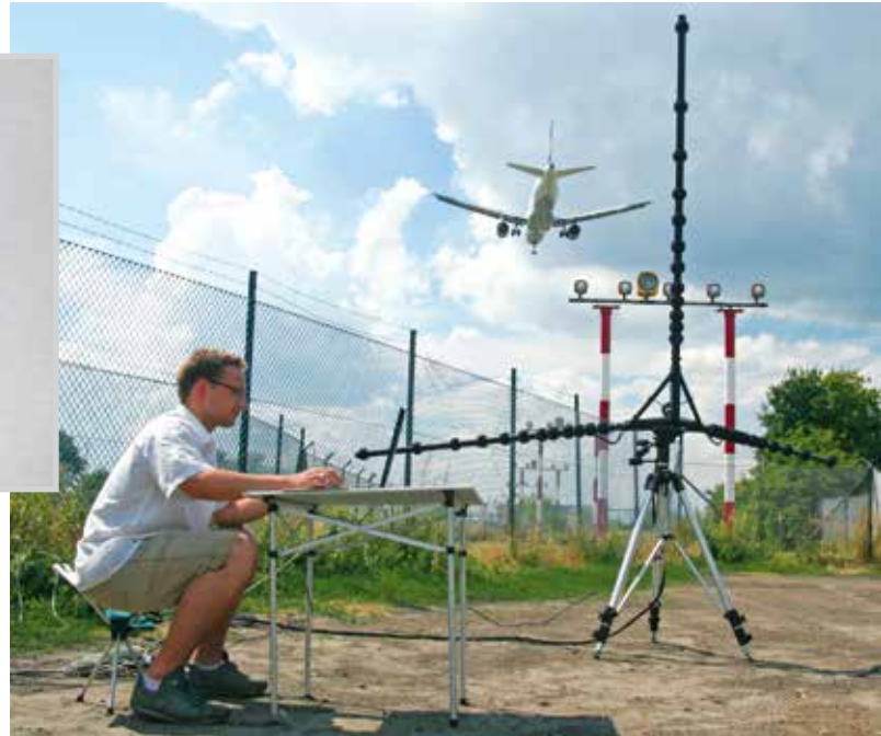
• • • Noise radiation from aircraft engines, gear and flaps and Acoustic Movie 2D.
