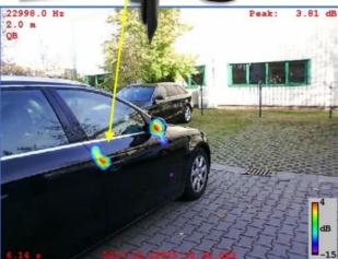
Sound Source located at the centre the of vehicle, white noise 20kHz-25kHz
