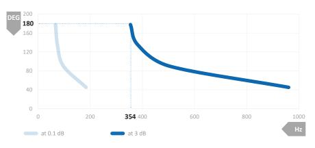
Calculation of the lowest frequency (Hz) at 180° opening angle (DEG)
