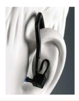
Take caution whenever the microphone is placed inside the human ear. Correct position for probe placement is the entry of the ear channel **not inside of it!**Otherwise sudden movements of the user or unexpected blows around ear area may cause serious injuries if enough carefulness is not kept.
