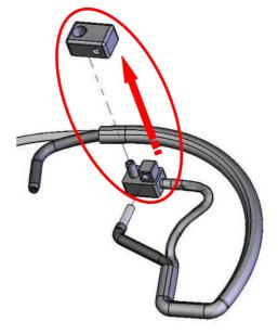
**Step three:** place the microphone probe (D/F) on the connector making sure that <u>one</u> o-ring (B) is placed between probe and connector. In a new set the o-ring is already mounted on the connector.
