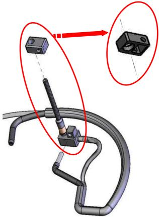
**Step five**: connect the ending of the over-ear microphone to the side hole of element A.
