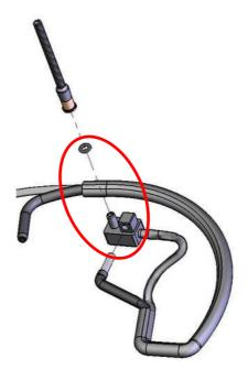
**Step four:** mount the microphone housing (A) on the probe putting the probe through the hole on the top of element A.
