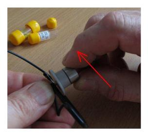
Press the microphone lightly with finger during the calibration:
