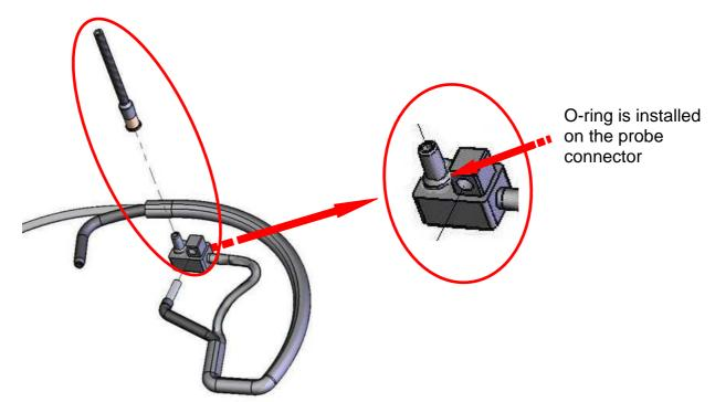
Use the spare o-ring only in case the original one is not placed on the connector:
