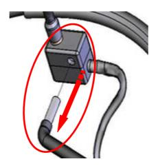
**Step two:** dismount the microphone housing (element A) from the over-ear microphone (K).
