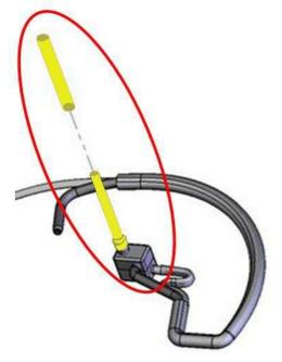
Before placing the SV 25S microphone in the ear remember to put the silica pipe on the probe.
