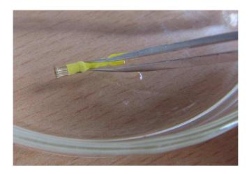
After washing in alcohol, the probe should be dried with compressed air:
