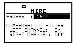
In order to choose the appropriate compensation filter, user has to select the **PROBES length** in the menu SETUP\MIRE and press the <ENTER>.
