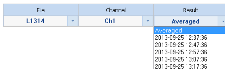
Fig. 5-20. Selecting a single Summary result or averaged results in the Hearing protectors panel
