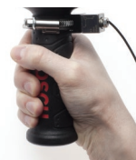
SV 150 Tri-Axial Hand-Arm Vibration MEMS Accelerometer
