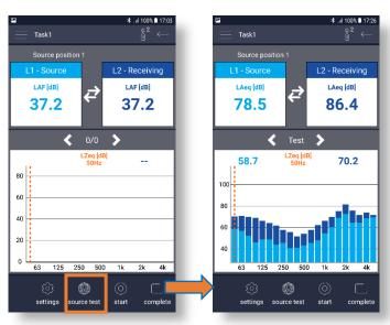
Having two measuring instrument you can perform measurements simultaneously in the source and receiving rooms.
