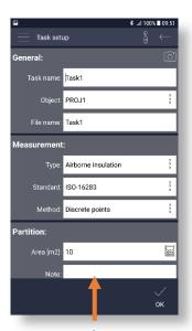
While creating new Building Acoustics task in the **Task setup** screen you should select one of the next task types in the **Measurement** section: *Airborne insulation, Facade, Impacttapping machine* or *Impact-rubber ball*.
