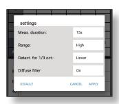
Tapping the icon in measurement screen, you can check or change the measurement settings: **Measurement duration** (1÷60s, Inf or Auto), measurement **Range** (High or Low), **Detector for 1/3 octaves** (Linear, Fast or Slow) and **Diffuse filter** (On or Off).
