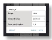
Tapping the (icon in measurement screen, you can check or change the measurement settings: measurement Range (High or Low), Ambient noise and Source calibration.
