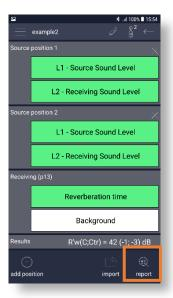
When all sound level measurements in the source and receiving room for all source positions are done and complete and reverberation time measurements complete, you can generate a report tapping on the active icon and selecting the report type - based on apparent sound reduction index R' or on standardized level difference DnT.
