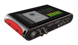
de- vice, that allows one to gain understan- ding about the sound field by listening, led to the development of Voyager. In addition, it offers real-time visualiza- tion, recording and audio filtering. The embedded touch controlled software offers the ability to run targeted vi- broacoustic analysis intuitively on the spot, monitor soundscapes and locate sound sources reliably over with quick scans.
