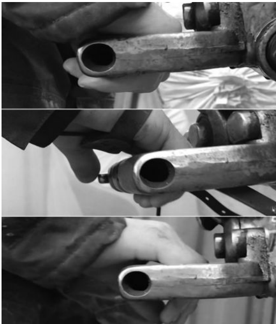
Figure 2. Type 1–3 hand grips (from top to bottom respectively). Top: closed grip with fingers and palm flexed around tool handle. Middle: semi-open grip with only fingers flexed around tool handle (no contact between tool handle and accelerometer). Bottom: open grip.
