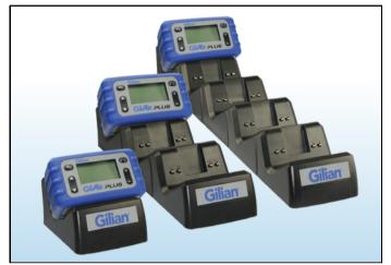
Three and five-station docks are included when ordering multi-pump configurations.
