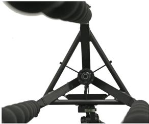
Aluminium array-body diameter: 3,4m
