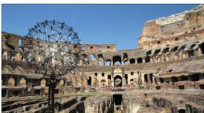
This spherical 120 channel microphone array is primarily designed for applications in enclosed spaces. Depending on a signal's spectral composition, the recommended measurement distance varies between 0.5 and 25 meters. Longer ranges are possible for measurements in considerably higher frequency ranges.
