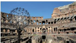
This spherical 80 channel microphone array is primarily designed for applications in enclosed spaces. Depending on a signal's spectral composition, the recommended measurement distance varies between 0.5 and 25 meters. Longer ranges are possible for measurements in considerably higher frequency ranges.
