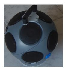
The DL103 is a smaller version of our usual dodecahedral sound source, providing omnidirectional excitation according to all the latest standards. The source can be driven from a sound level meter, or an internal noise source that has been equalised for a flat response over the complete frequency range.
