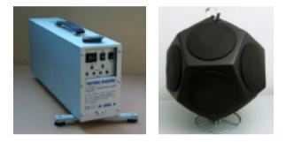
Their noise sources include the EM50 Tapping Machine which uses an electromagnetic technique to drive the hammers; a totally silent method so no more mechanical cams rattling around causing noise and wear. Their dodecahedral sound source provides omnidirectional excitation according to all the latest standards. It can be driven from an external device like the SoundBook or an internal noise source that has been equalised for a flat response over the complete frequency range.
